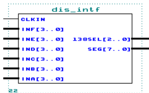
Figure 7.19c The internal circuit symbol of scan display circuit
