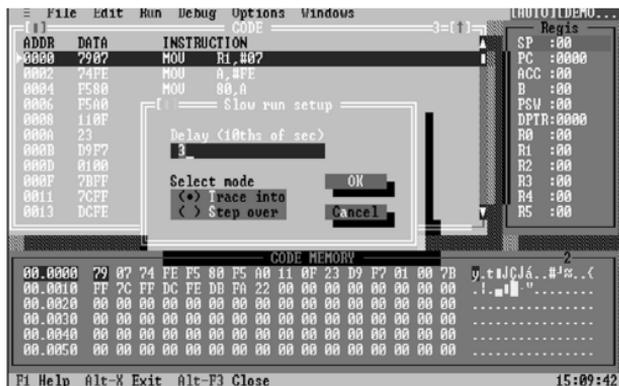
\*Delay (10ths of sec): Set the delay time for the program running. The minimum is 1 and the maximum is 50.
