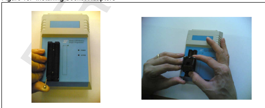
Figure 10. Installing Socket Adapters
